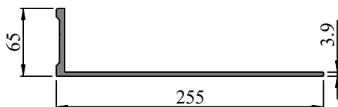
SEC. NO. FW0010 WEIGHT - 3.643 Kg/M
